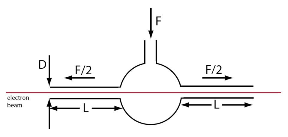
T=15 K, F = 1.5 x  $10^{18}$  s<sup>-1</sup> (100 mTorr-liter per sec), L= 10 cm, D = 2 mm Target thickness =  $10^{19}$  cm<sup>-2</sup>
